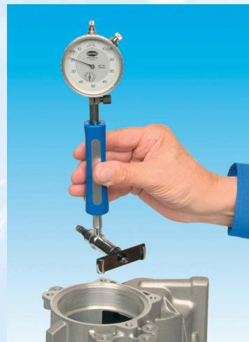
Features of the indicating 2-point gauges are easy handling, adaptability to most bore gauging applications and large measuring ranges. Calibration (zero setting) can be easily made in a micrometer by using the DIATEST setting guide or in a setting ring. Gauge automatically self-centers via a centering bridge.
